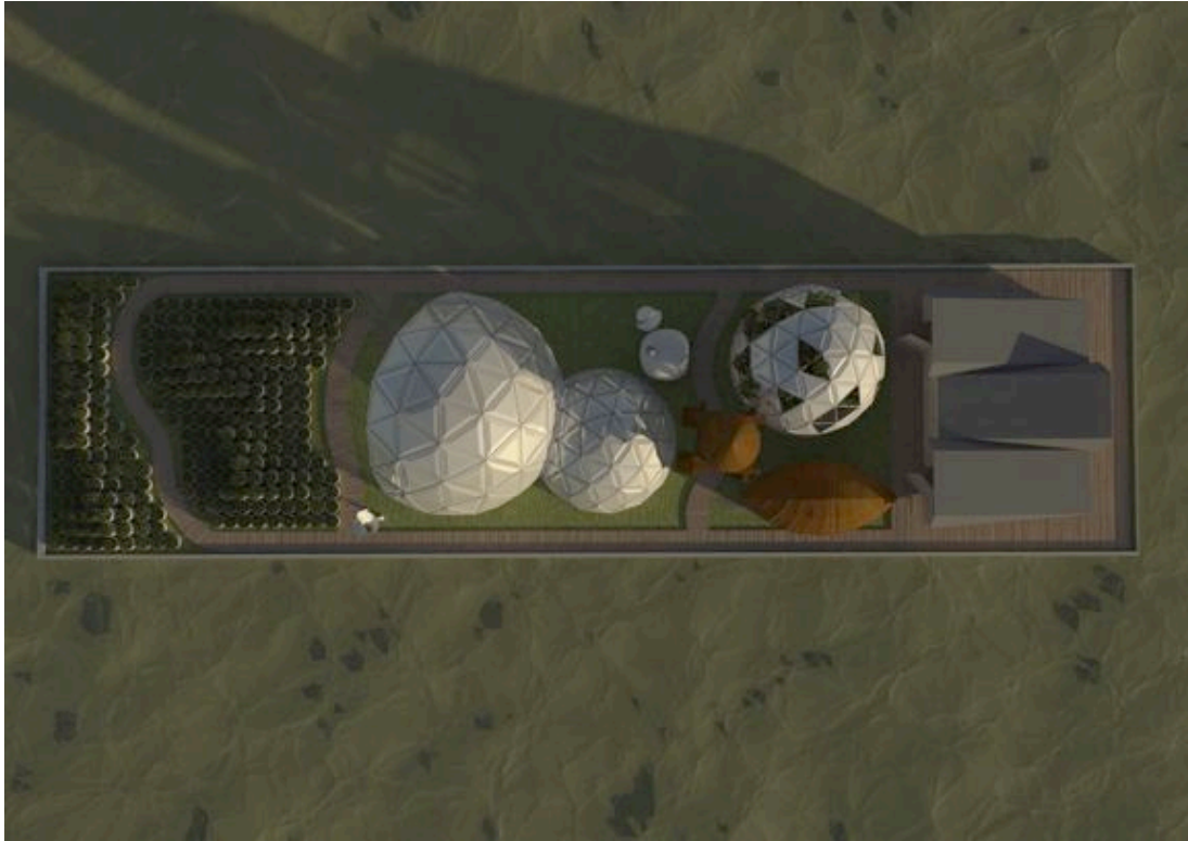
Image 1. Waterpod™ from Above, showing from Left to Right: Gardens; Public space; Workspace, Composting Toilet; Watertower; Kitchen/Shower facility; Garden sphere; and living accommodations.
